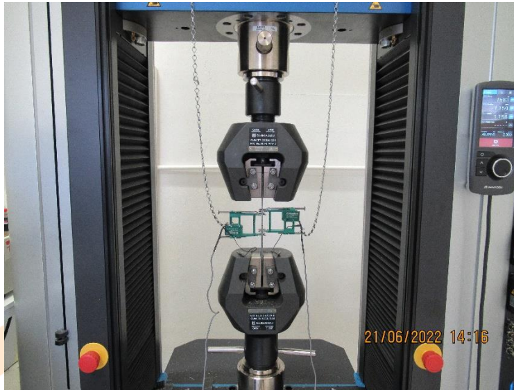
Figure 1. Photographs of sample EHC plate, test specimens & Shimadzu tensile test machine
