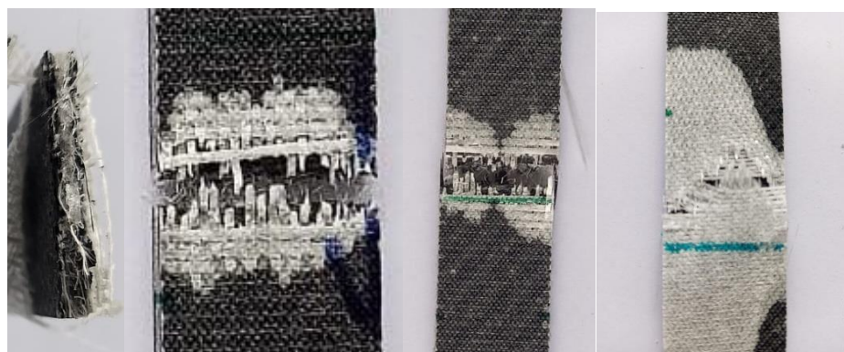
Fig. 4 The damaged digital sample photographs after the tension tests
