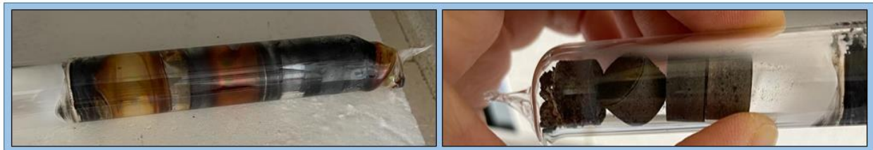
Figure 4. Composite materials sintered in a quartz tube
