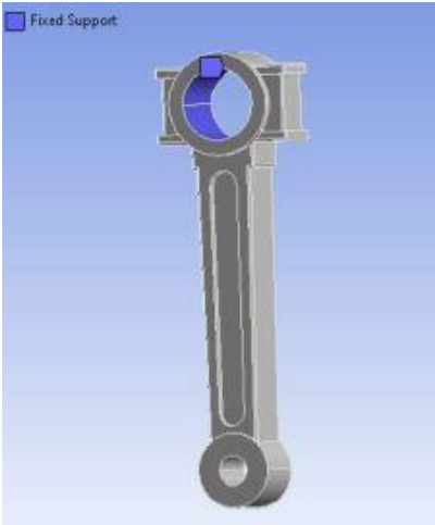
Figure 2. Fixed support region for design
